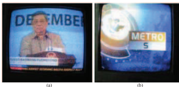
Fig.10: The quality of TV trainer reception using an L-dipole antenna
